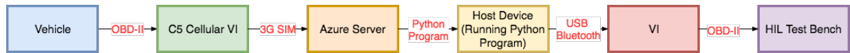
Figure 6: A top-level architecture diagram depicting the transmission of a CAN message from the data collection vehicle to the HIL test bench, to allow for virtual remote access to the vehicle.
